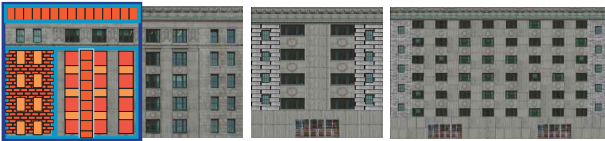
Figure 15. Left: The original facade picture partially overlaid with the grid structure, where blue frames and red grid cells are nested and random image layers, respectively. Middle and right: Two facades in that style at different sizes.
